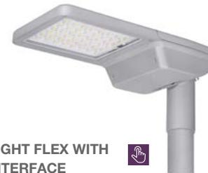
Modular lighting with ZHAGA interface in durable design and highest quality components for long lasting performance for future proof, SMART CITY area lighting and M-, C- and P-class roads acc. to EN 13201. IP66, IK08, SK2, very long lifetime (L90/B10): up to 100 000 h, spigot for 42, 48–60 and 76 mm poles available, tool-free housing opening and pushbutton terminal, no Upward Light Output Ratio (ULOR 0 %) when mounted at 0° tilt.
