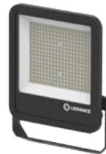
Highly versatile, asymmetric and robust floodlight with Power Select. For various outdoor applications and special tasks thanks to D-Mark certificate. Energy savings thanks to system efficacy of up to 130 lm/W, increased sea salt resistance with up to 480h, IP65, IK07 or IK08 (>6 000 lm), lifetime of 75 000 h (L80/B10), 1 m cable for perfect and easy connection.
